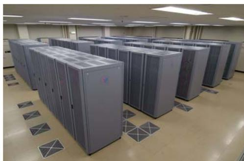
with single core, to provide the best balance between CPU FLOPS and memory bandwidth as well as network bandwidth. The parallel processing network consists of 6-way trunked Gigabit Ethernet in very unique 3-D HyperCrossbar topology.
